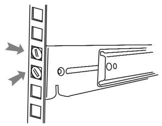
Figure 50 Attach Outer Rail and Slide Chassis in
